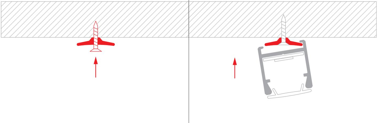
**NOTE!** Unusual dismounting of the extrusion. Move the extrusion in one of the directions in the horizontal plane, gently pull one side of the extrusion down, and remove the extrusion from the brackets.
