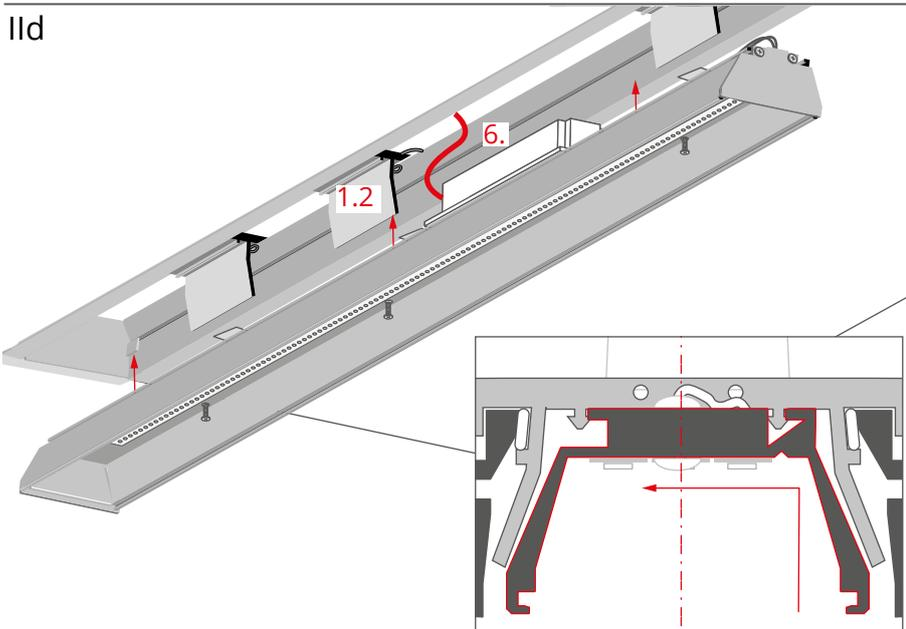
Connect the main power cables to the power supply (6).
