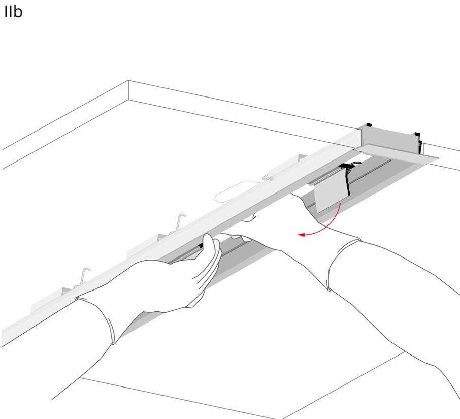
Lock the springs (1.4) at each item (1.2) by turning them, pressing them against the plate surface and sliding under the edge of the item (1.2) as shown in the figure.
