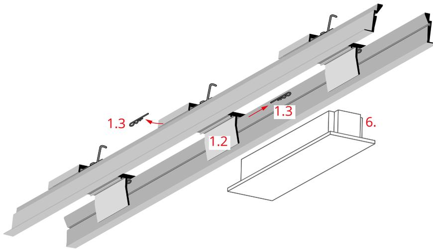
If the power supply (6) does not fit into the openings of the RAM-KOL-50 profile, its items (1.2) must be slid further apart accordingly.
