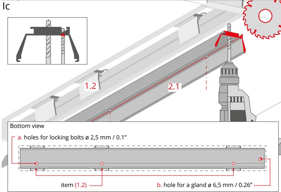
a. Drill holes for locking bolts in the profiled orientation line in the profile (2.1).
