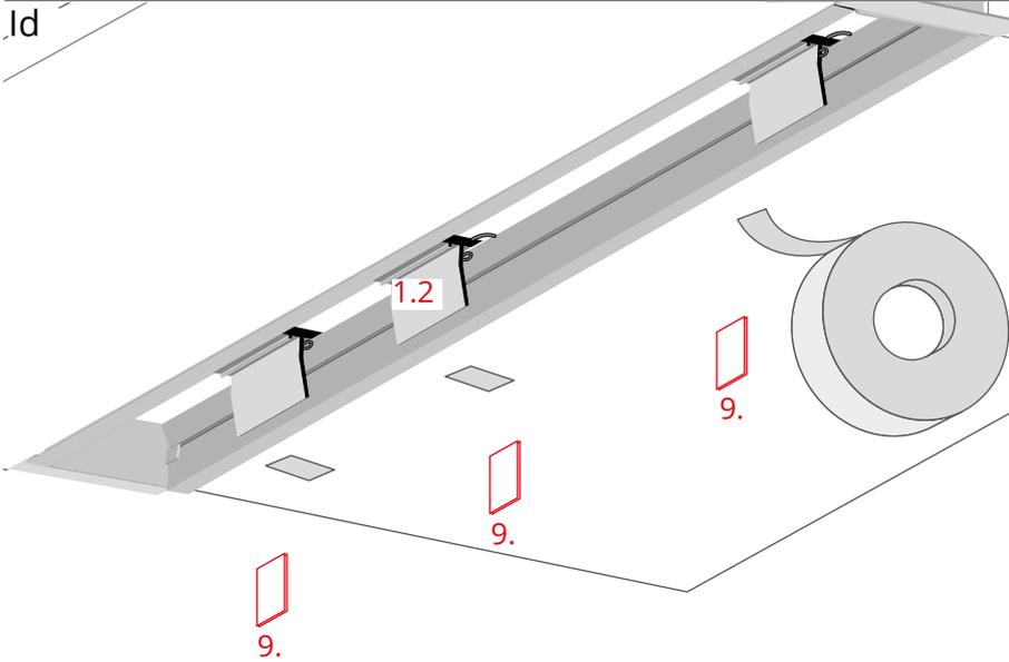
To facilitate further work, mark the location of the items (1.2) in the RAM-KOL-50 profile, e.g. with colored adhesive tape.
