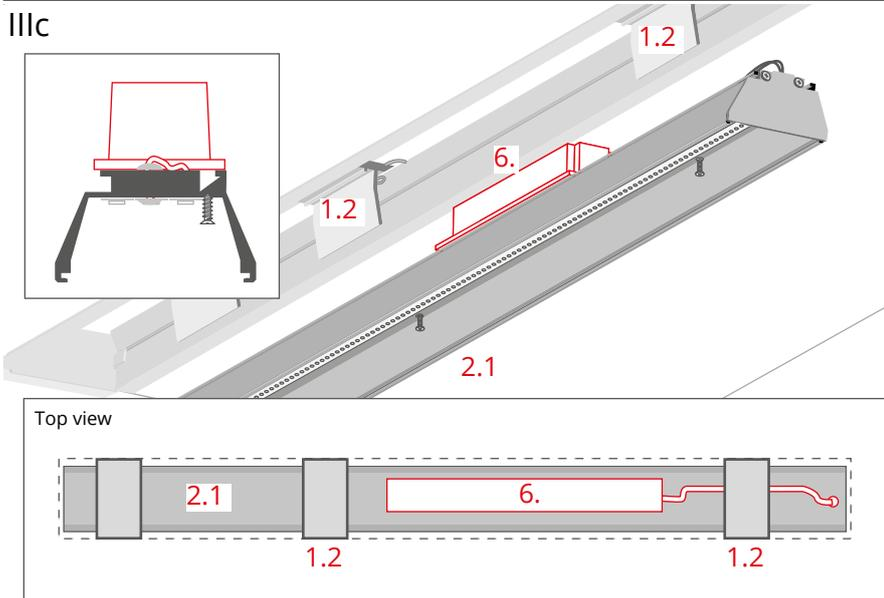
Mount the power supply (6) on the back of the profile in such a position that it fits into the opening of the RAM-KOL-50 profile.
