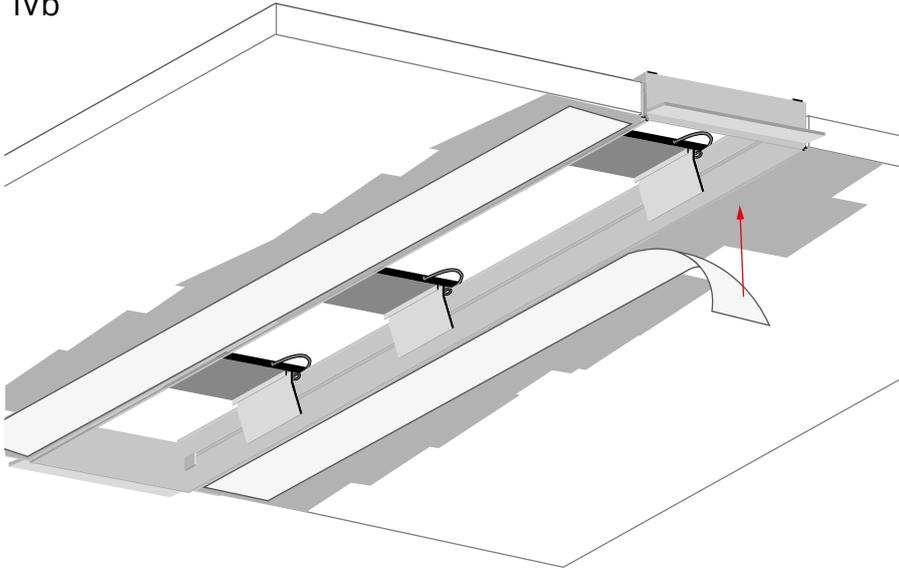
Attach TUFF-TAPE or equivalent at the junction of the profile flanges and drywall.
