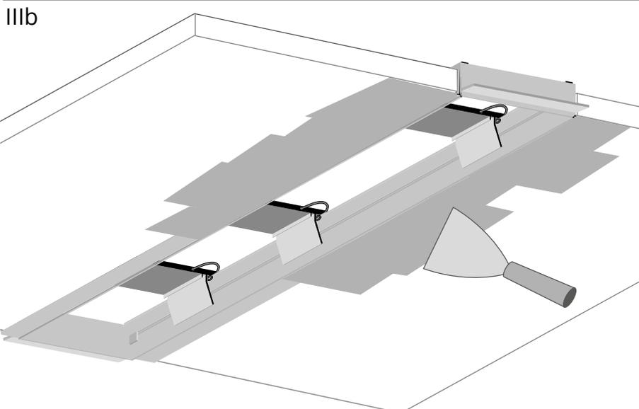
Apply glue and spread it at the junction of the profile's flanges and drywall.
