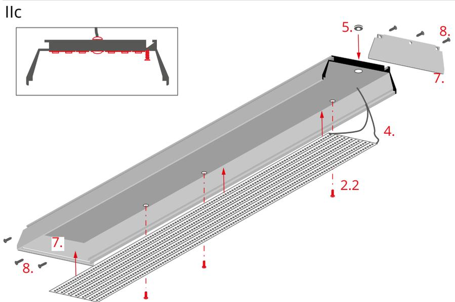
Adhere the LED tapes (4), mount the gland (5) and route the power cable through it.
