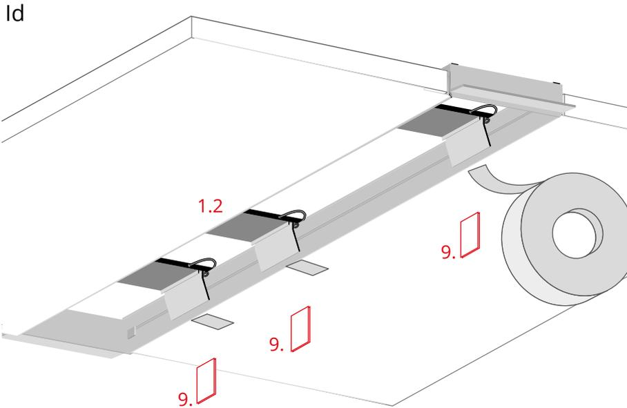
To facilitate further work, mark the location of the items (1.2) in the RAM-KOZE-100 profile, e.g. with colored adhesive tape.
