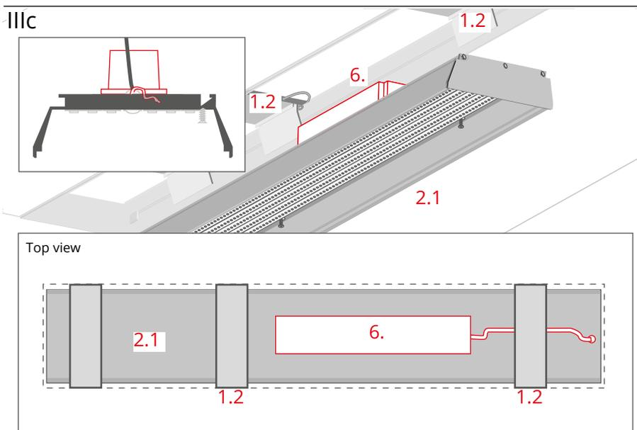
Mount the power supply (6) on the back of the profile in such a position that it fits into the opening of the RAM-KOZE-100 profile.
