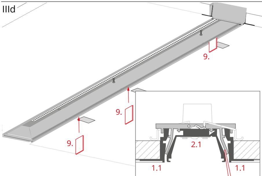
To prevent the OMODO-50 profile from falling out, insert wedges temporarily (9). They should be inserted into the marked spots in the gap between item (1.1) and item (2.1). There should be one wedge for each marked element (1.2) and they should be placed from the side of the profiled orientation line.
