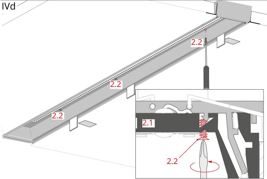
Secure the item (2.1) against slipping out by tightening the locking bolts (2.2) in the pre-drilled holes.
