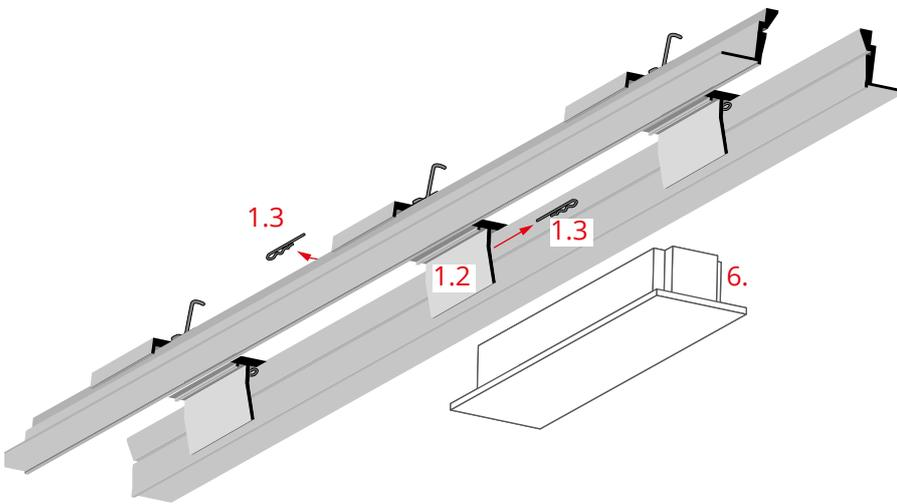
If the power supply (6) does not fit into the openings of the RAM-KOZE-50 profile, its items (1.2) must be slid further apart accordingly.
