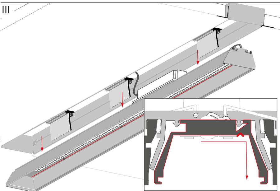
Slide the OMODO-50 profile towards the profiled orientation line and pull it down (as shown in the figure).
