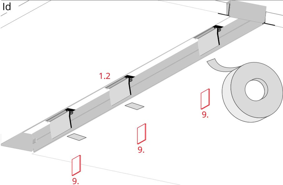
To facilitate further work, mark the location of the items (1.2) in the RAM-KOZE-50 profile, e.g. with colored adhesive tape.
