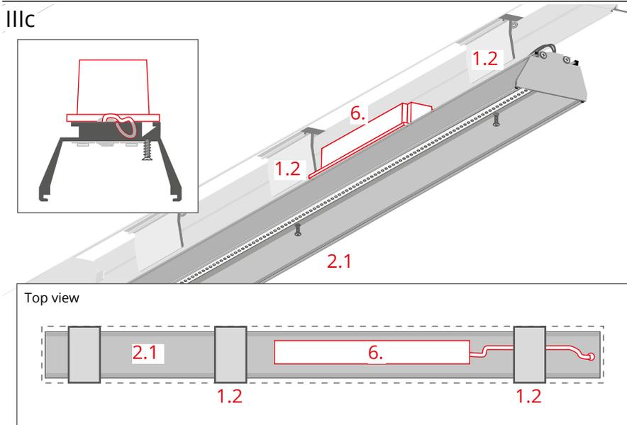
Mount the power supply (6) on the back of the profile in such a position that it fits into the opening of the RAM-KOZE-50 profile.
