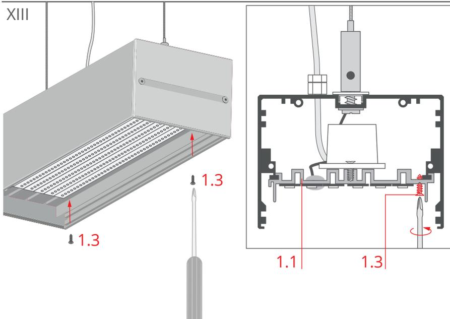
Secure the extrusion item (1.1) against slipping out by screwing the locking bolts (1.3) into the pre-drilled holes.
