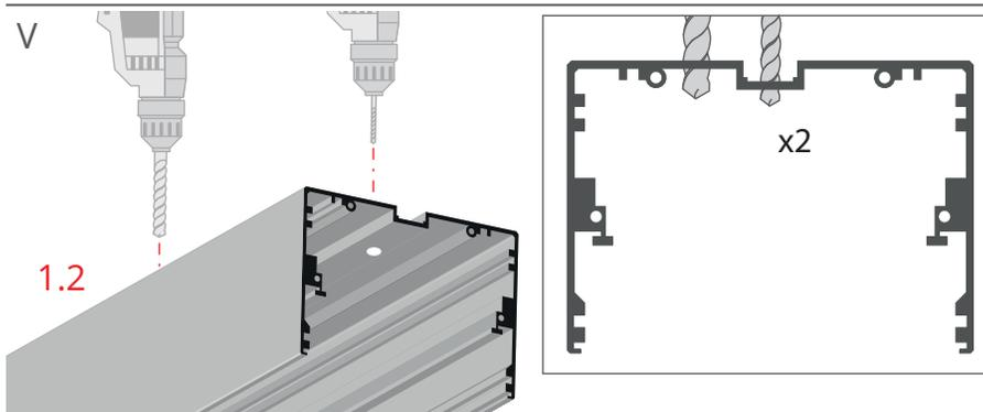
a. Drill two holes for the fasteners in the channel on the back of the extrusion (1.2). They do not have to be in a specific location.
