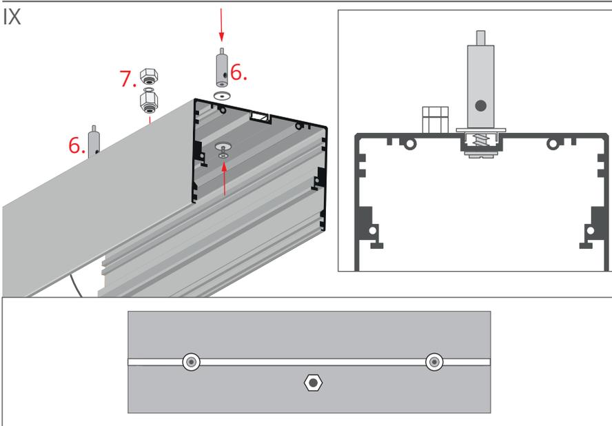
Attach the fasteners (6) and mount the metal gland (7).
