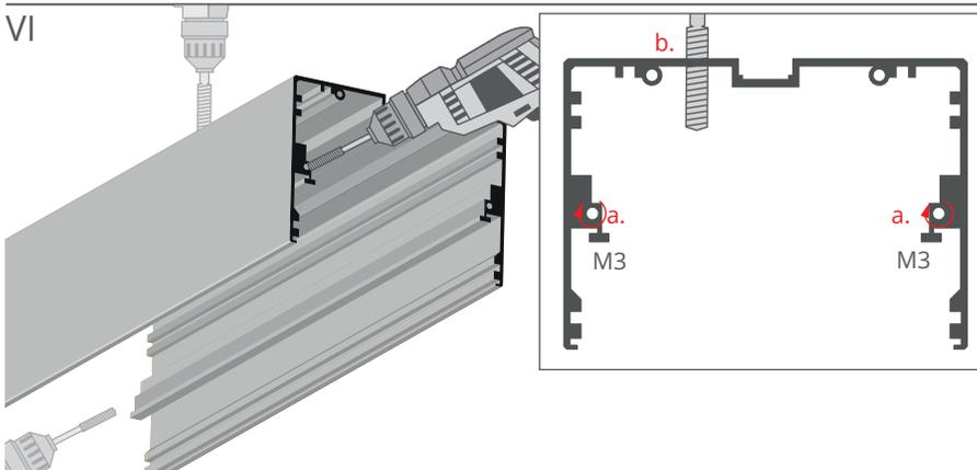
a. On both sides, from the side of the profile cross-section, thread the sockets for end cap bolts to a depth of approx. 15 mm / 0.59". (M3 tap)
