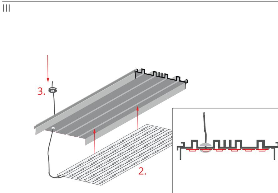
Install the LED tapes (2), insert the gland (3) and feed the power cable through it.
