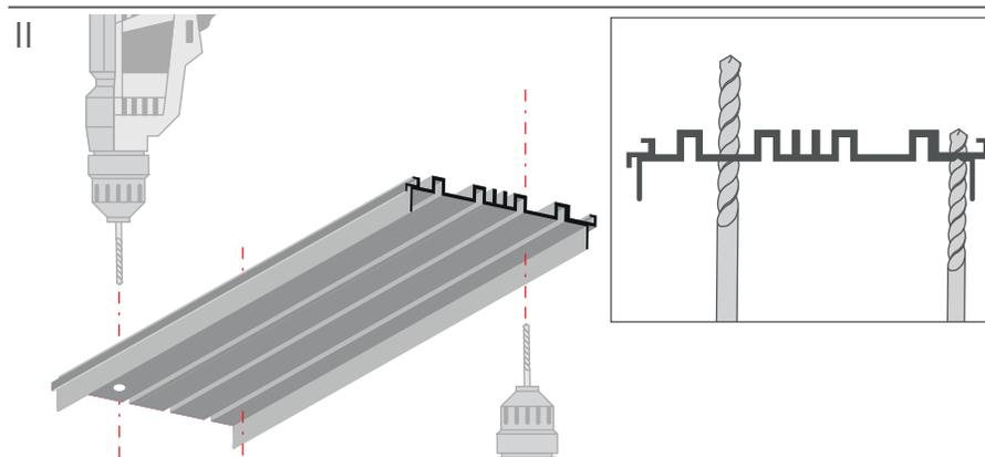
a. Drill holes for locking bolts in the profiled auxiliary line. The required number of holes is:
