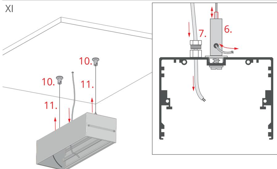
Fasten the extrusion on steel wires (11) to the ceiling fasteners (10). The suspension length can be adjusted by pressing the upper part in the fastener body (6).
