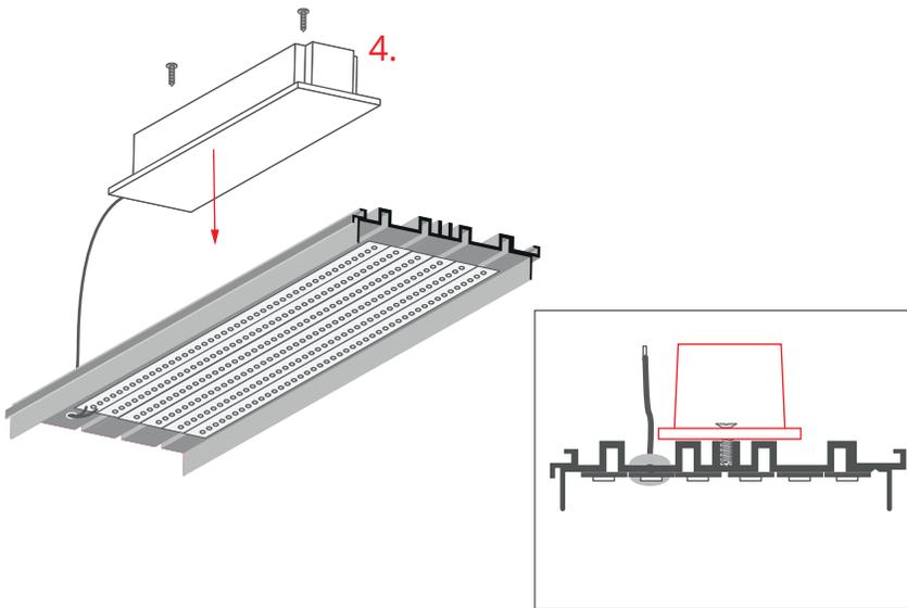
Mount the power supply (4) on the back of the extrusion.
