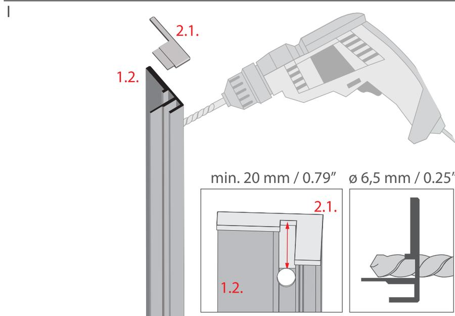
Drill a hole 6.5 mm / 0.25" in diameter in the KRAV-05IN profile (item 1.2) for the power cable.
