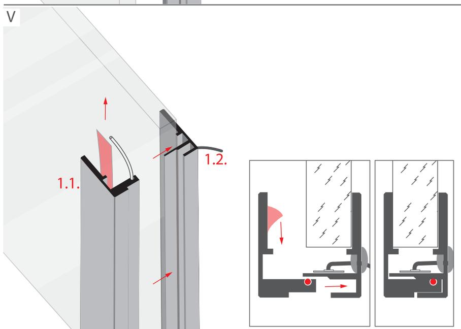
Peel off the red protective foil and glue item (1.1) to the edge of the glass or plastic as shown in the drawing.
