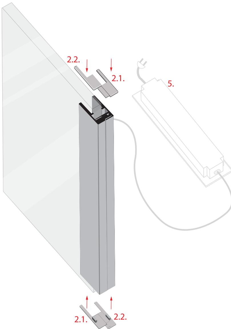
Put both end cap parts on both ends of the profile. First insert item (2.1), then item (2.2).
