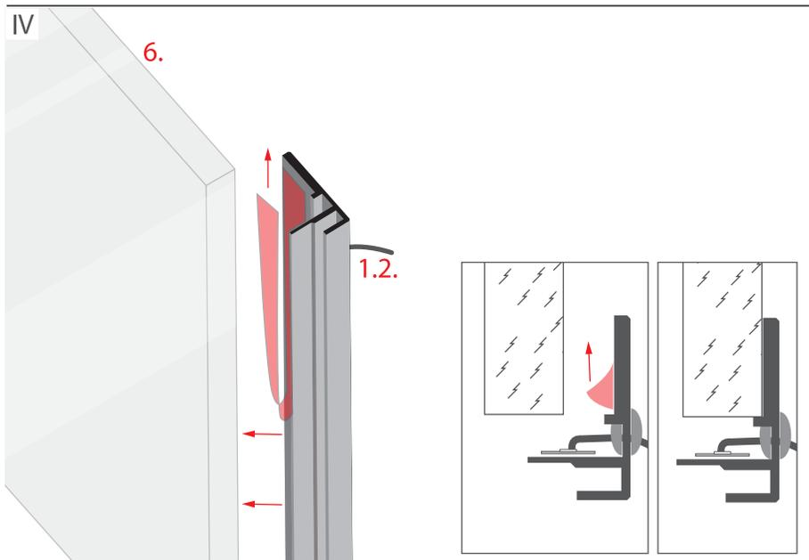
Peel off the red protective foil and glue item (1.2) to the edge of the glass or plastic (6) as shown in the drawing.
