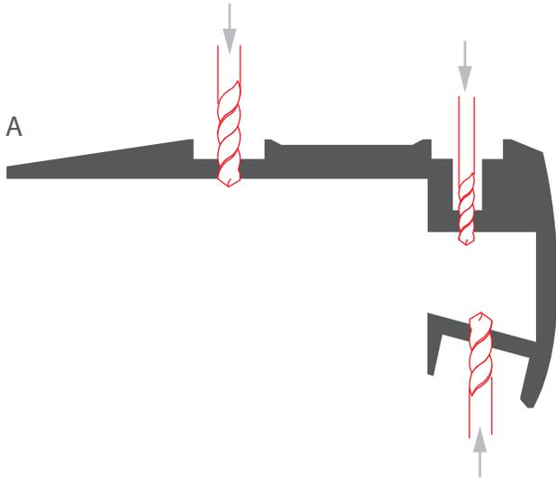
**2.** Attach the LED strips (C) and lead out the power cable. Next mount the extrusion (A) to the step with suitable screws.
