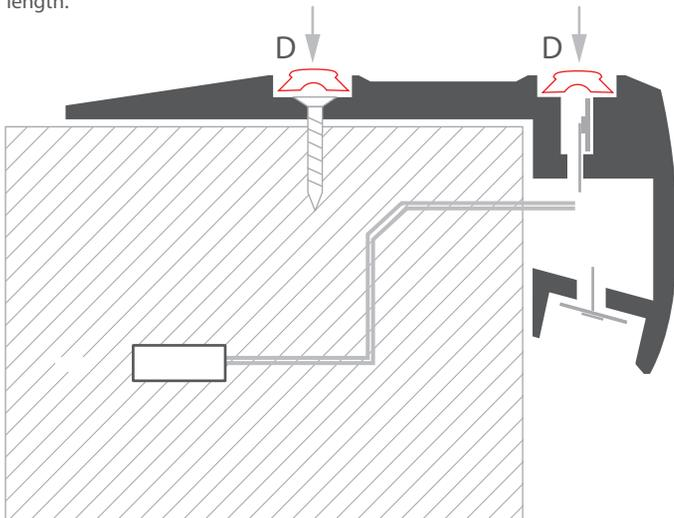
**4.** Mount the cover (E) and connect the LED strips to the power supply.
