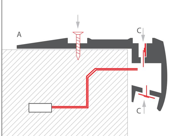
**3.** Insert anti-slip rubber strips (D) into the extrusion. To do this, stretch the strip slightly or use a slippery substance. **NOTE:** After inserting the strip in the extrusion do not cut the excess length! It will slowly spring back to its former length.
