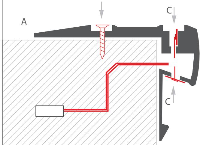
**3.** Place the non-slip strips (D) into the grooves. To do this, slightly stretch the non-slip strip or use a slippery substance. **NOTE:** After placing the anti-slip strip in the extrusion do not cut it as it will return to its original length on its own.
