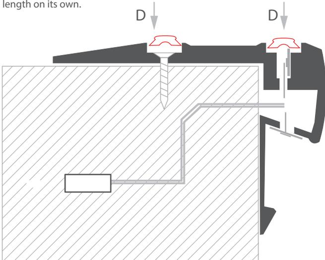
**4.** Snap in the cover (E) and connect the LED strip to the power supply.
