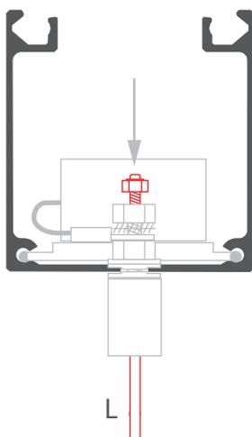
**10.** Insert the extrusion (B) into the mounting strip (A) and connect power.
