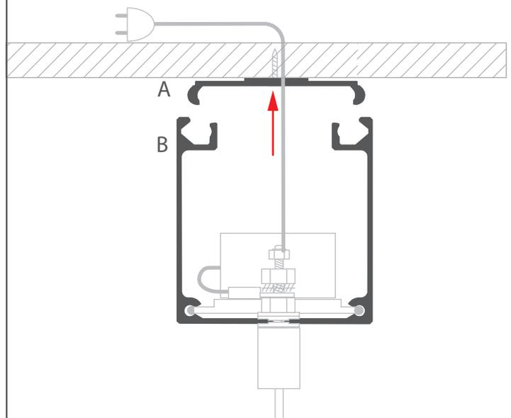
**11.** Secure the extrusion (B) against falling off by inserting the 4mm plastic rods (H) into the guides and tightening them with M5 pressure screws (I) using the Allen wrench. Sink the pressure screws deep enough so there is room for end caps.
