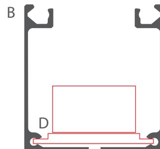
**7.** Secure the power supply bracket (D) with the power supply by inserting one 2.4 mm plastic rod (G) into the guides on each side. Cut the rods to the required length. Next secure the rods with M3 pressure screws (J), tightening them with the Allen wrench.
