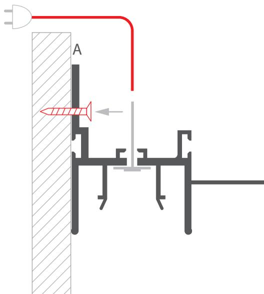
**4.** Insert the hook of the stretched ceiling (D) into the extrusion (A).
