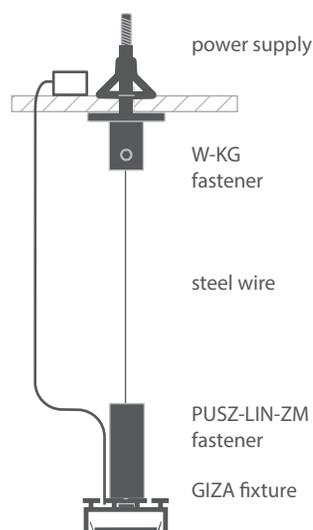
**4) Wire - Rod - conductive driven power supply**
