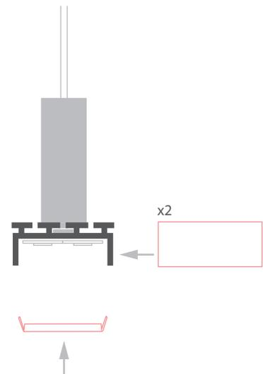
**5.** Install the W-KG-Z ceiling fasteners. The fastener installation manual can be downloaded at [www.klusdesign.eu](http://www.klusdesign.eu). Connect the cables, each for the single power pole to the fasteners. The cables should go through a pre-drilled hole just under the masking cover of the fastener.
