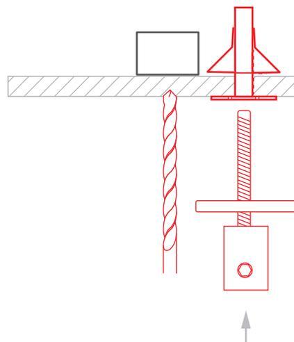
**6. Mount the fixture with steel wires into the ceiling fasteners.** Connect the cable to the power supplier, leading it through a pre-drilled hole in the ceiling.
