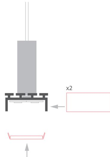
**5.** Install the W-KG ceiling fasteners. The fastener installation manual can be downloaded at [www.klusdesign.eu](http://www.klusdesign.eu). Place the power supplier next to the fastener and drill the ceiling to lead the cable to it.
