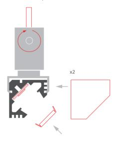
**6.** Mount the fixture with rods into the ceiling fasteners. Connect the powering cable.
