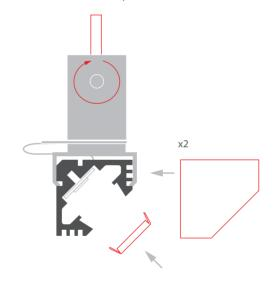
**6.** Mount the fixture with rods into the ceiling fasteners. Mind that the power poles connected to the rods should match the ones connected to the fasteners.
