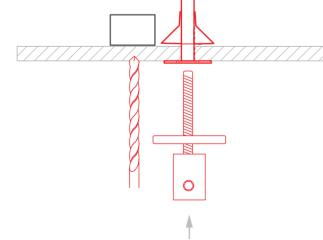
2. Insert the extrusion into the mounting bracket of the head. Manual for the DP-45-MOC fastener can be downloaded from www.klusdesign.eu.
