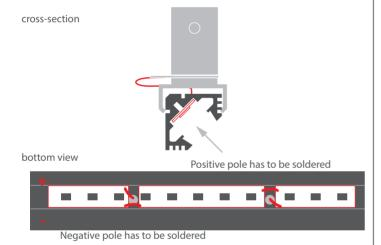
**5.** Install the W-KG-Z ceiling fasteners. The fastener installation manual can be downloaded at <a href="www.klusdesign.eu">www.klusdesign.eu</a>. Connect the cables, each for the single power pole to the fasteners. The cables should go through a pre-drilled hole just under the masking cover of the fastener.
