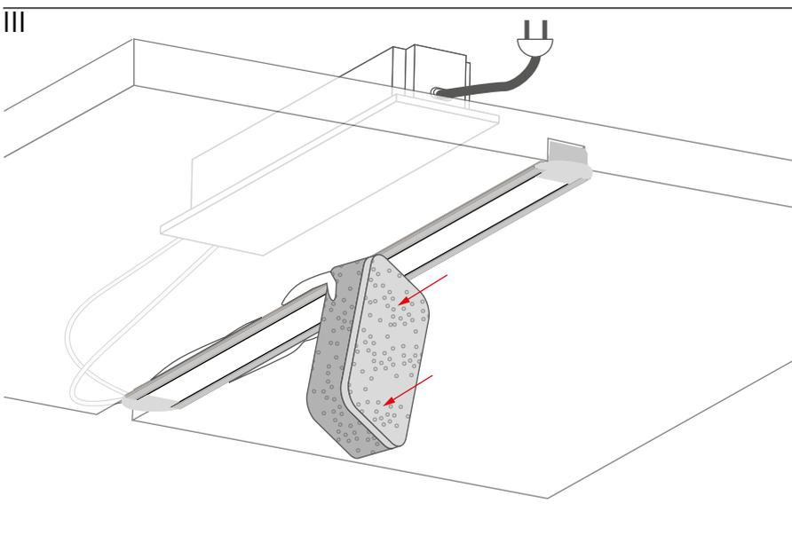
Remove the excess glue from the lighting fixture.
