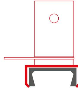
**3.** Mount the LED strip in the extrusion and lead the cables through pre-drilled smaller holes. Then lead them to the connectors of the DP-MOC-ZZ fasteners. Each hole should lead a cable with one power pole, LED strip has to be cut before installation, so the wires can be easily routed to the holes.
