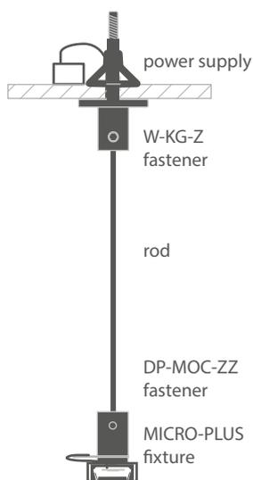
**2) Rod - non-conductive (drop lead)**
