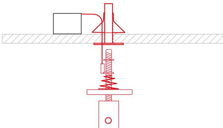
**6.** Mount the fixture with rods into the ceiling fasteners. Mind that the power poles connected to the rods should match the ones connected to the fasteners.
