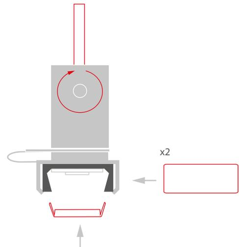
**5.** Install the W-KG-Z ceiling fasteners. The fastener installation manual can be downloaded at [www.klusdesign.eu](http://www.klusdesign.eu). Connect the cables, each for the single power pole to the fasteners. The cables should go through a pre-drilled hole just under the masking cover of the fastener.
