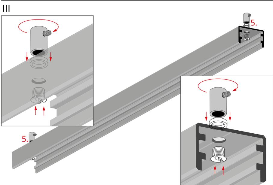
Screw the fasteners (5) to the profile.
