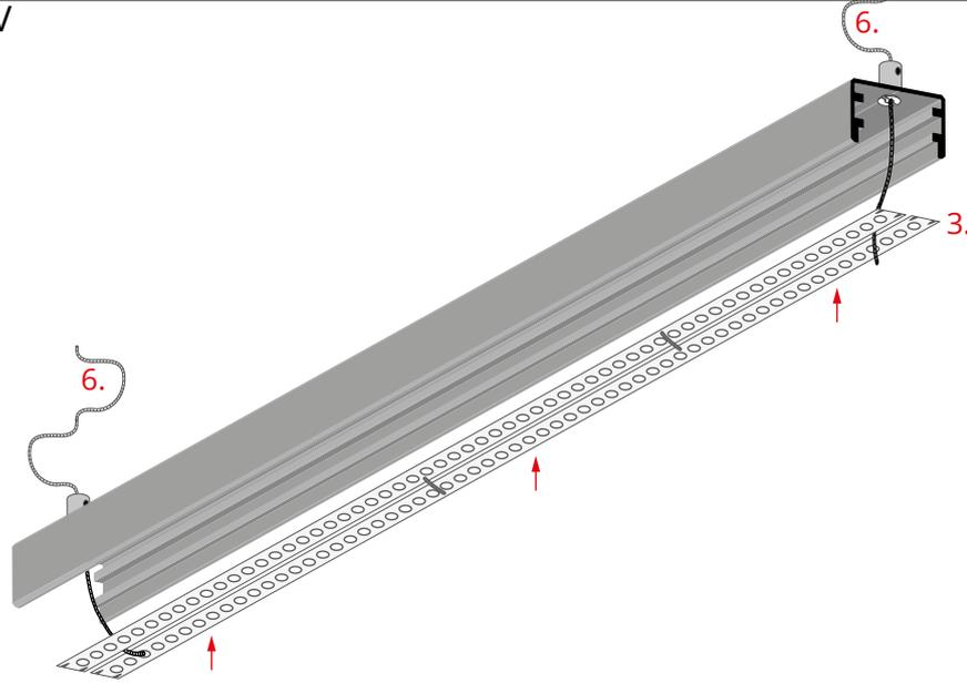
Run the cables (6) through the fasteners into the profile.
