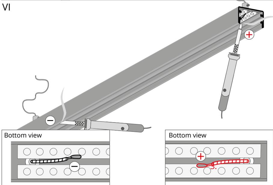
Solder the cable cores to the appropriate current poles.
