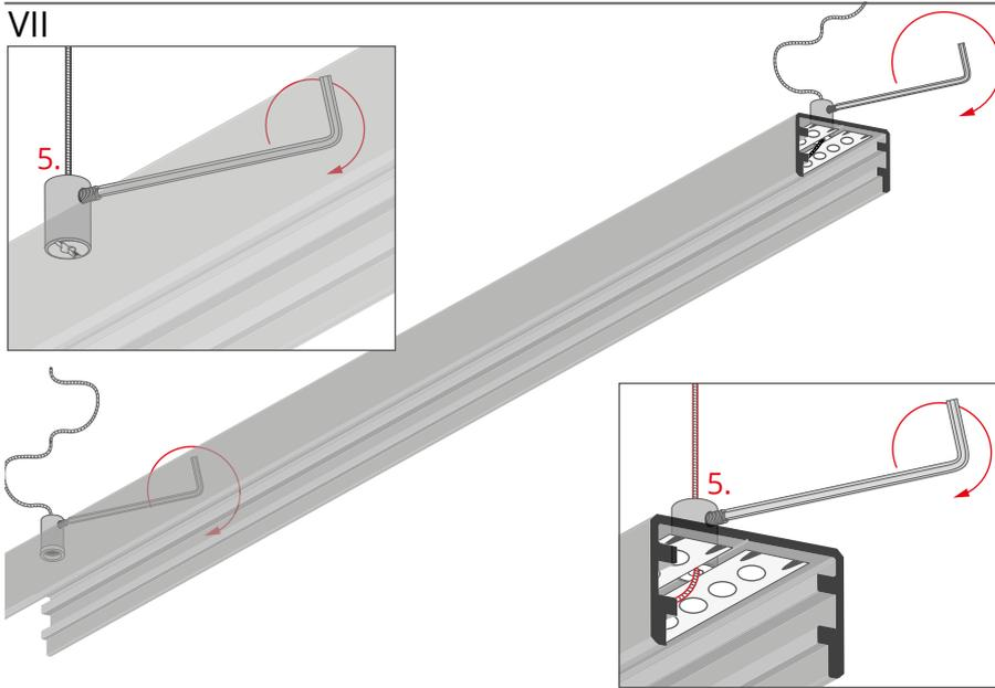
Lock the cables by tightening the pressure screws in the heads of the fasteners (5).
