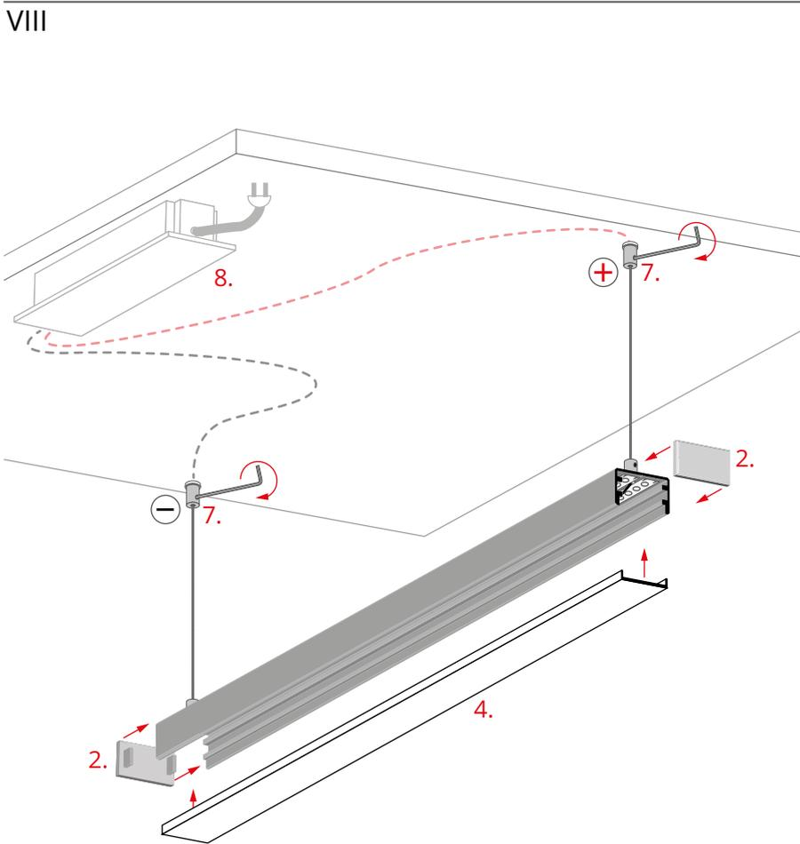
Mount the cover (4) and the end caps (2). Suspend the profile on the ceiling fasteners (7). Connect the 12 V / 24 V power supply (8) to the ceiling fasteners.
