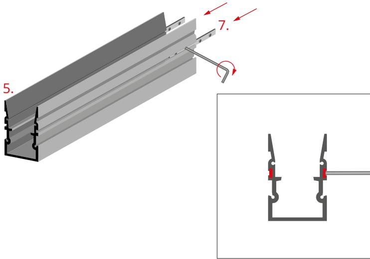
Place the ZM connectors (7) halfway in the HR-MAX-TW profile channels (5).
