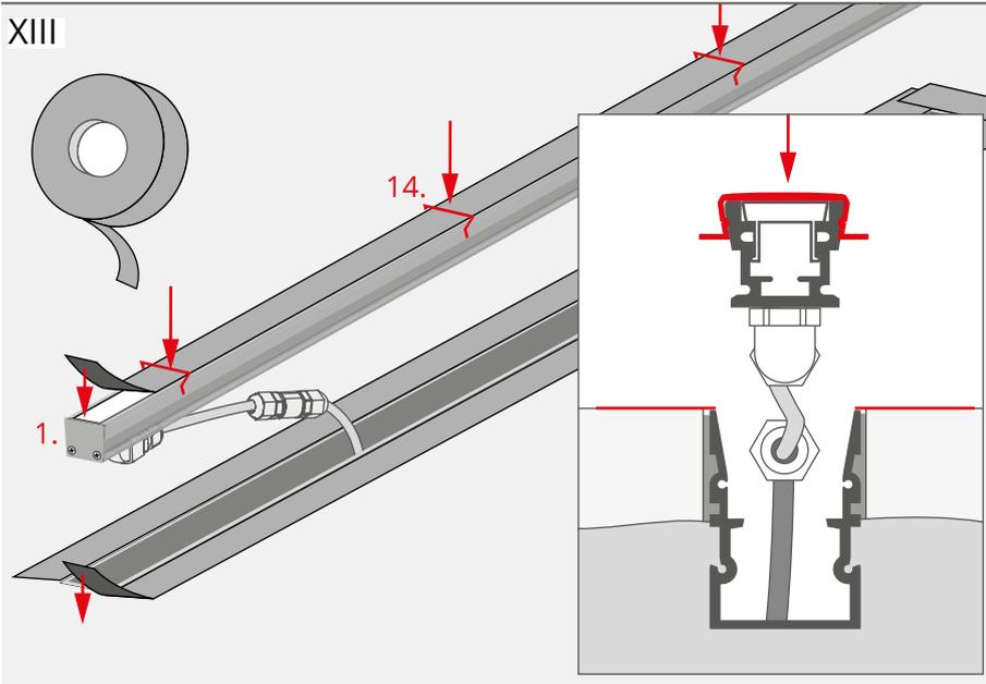
Secure the surface of the fixture and the edges of the mounting track with protective tape.
