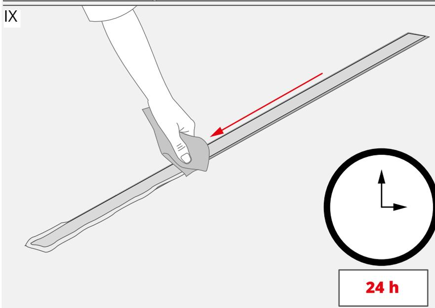
Remove the excess grout and wait 24 hours for the grout to dry.
