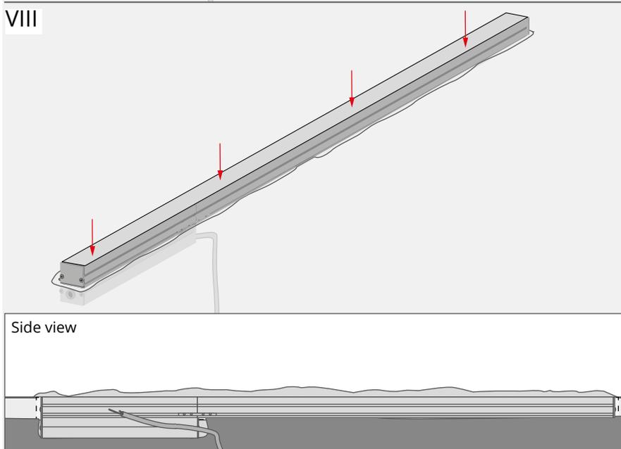
Insert the mounting track into the channel.
