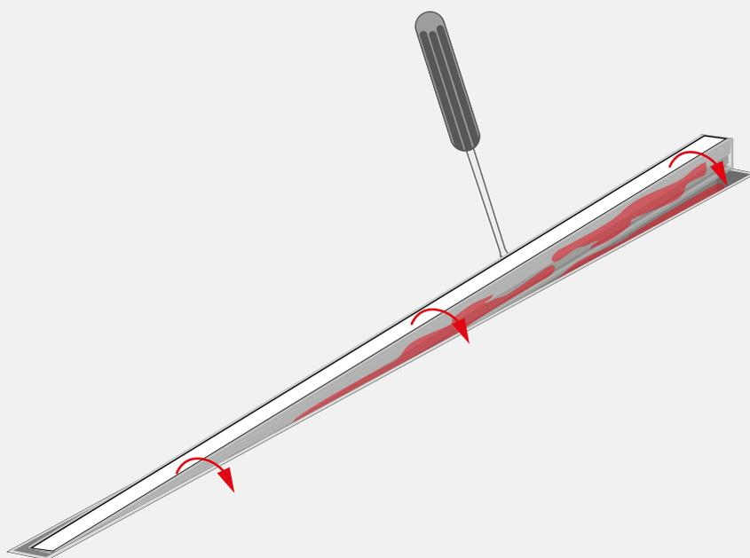
Using e.g. a flat screwdriver, pry up the fixture and remove it from the track.
