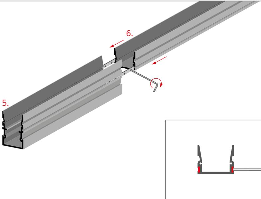
Use the ZM connectors to connect the HR-MAX-TW profile (5) with the HR-MAX-T profile (6).
