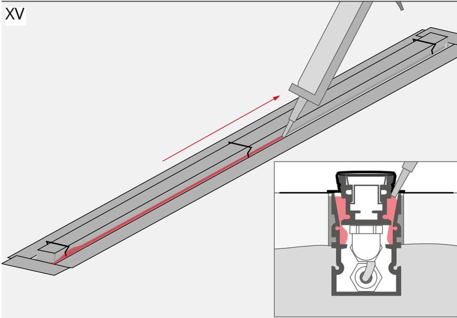
Put a portion of silicone into the space between the lighting fixture and the mounting track.
