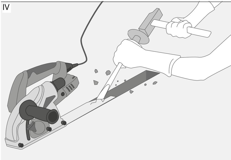
Cut a channel in the concrete base for the connected HR-MAX-TW and HR-MAX-T profiles.
