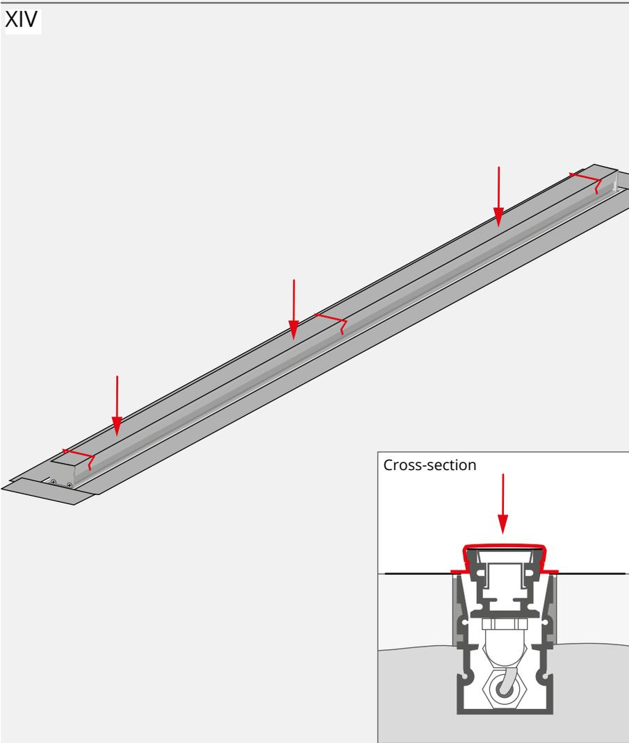
Insert the HR-MAX fixture together with the coupler and cable into the mounting track. The gland of the fixture and the coupler should be in the lower chamber of the HR-MAX-TW profile.
