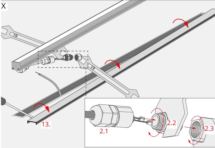
Remove the protective insert (13), by prying it out with a flat screwdriver.
