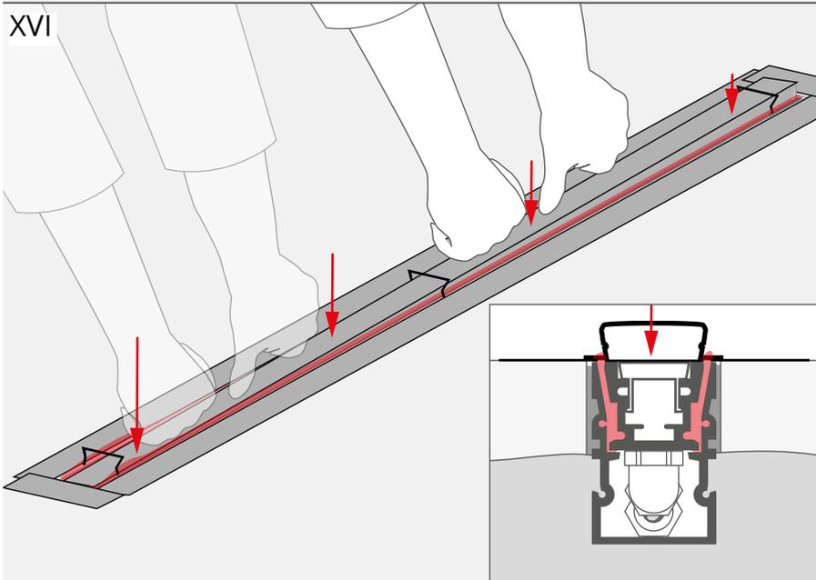
Press successive sections of the lighting fixture down, so that they reach the bottom of the mounting track.
