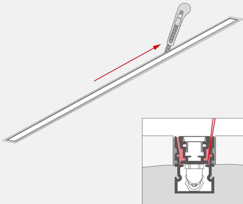
To disassemble the lighting fixture, use a knife to cut the layer of silicone between the wall of the fixture and the mounting track.
