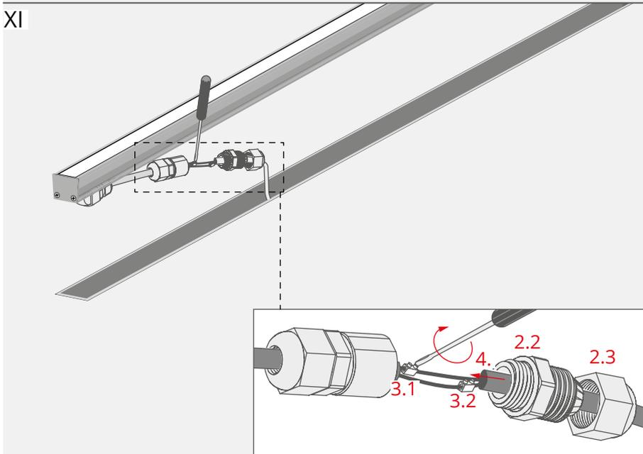
Lead the cable (4) through items (2.2, 2.3) of the hermetic coupler and attach it to the cable from the fixture, using both items (3.1, 3.2) of the connector.
