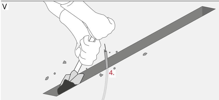
Create a recess for the HR-MAX-TW profile. In it, lead out the cable for the 12 V / 24 V power supply (4).
