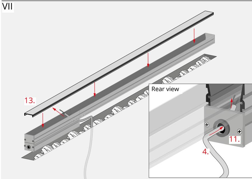
Mount the protective insert (13) in the mounting track made of the combined HR-MAX-TW and HR-MAX-T profiles.
