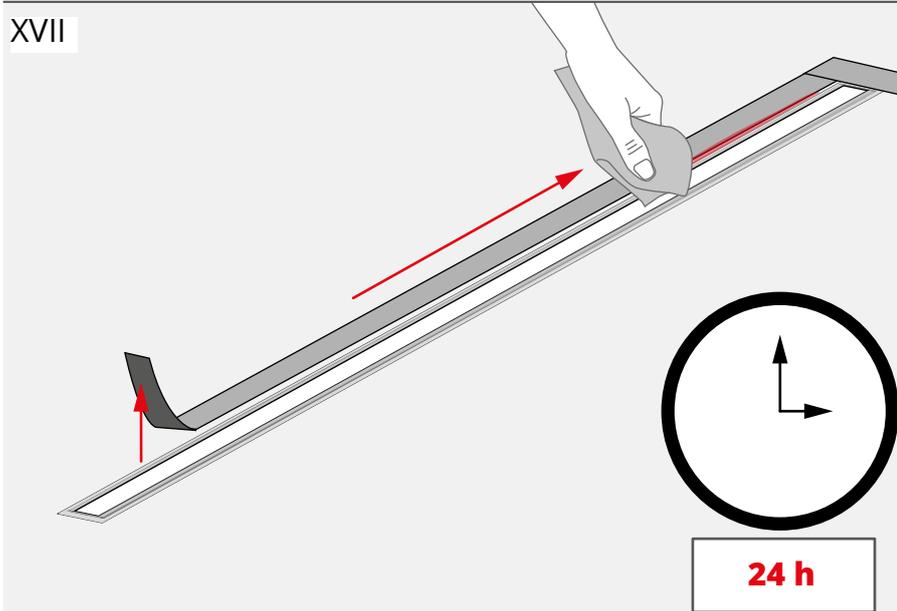
Remove excess silicone from the surface and remove the protective tape. Wait 24 hours for the silicone to dry.
