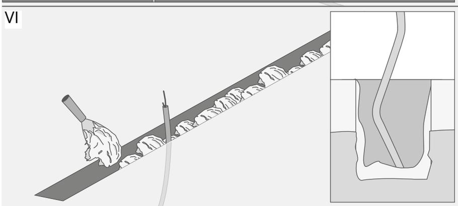
Apply a layer of grout to the walls and bottom of the channel.
