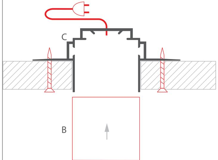
**3.** Slide the clips into the LED fixture, then connect power and insert the LED fixture into the extrusion (A). The number of clips should be: 4 for 1-meter long profiles, 9 for 2-meters long profiles and 14 for 3-meters long profiles. First and last clip should be placed 5-7 cm from the end of the profile.
