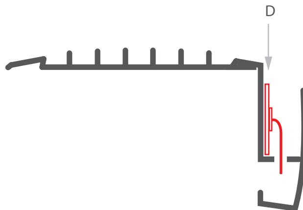
**2.** Fasten the extrusion (A) to the surface with appropriate screws for the substrate.
