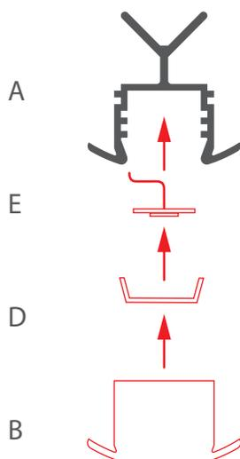
**2.** Feed the power cable and put the mounting insert (C) in the railing.
