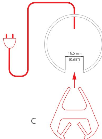
**3.** Connect power, and then mount the extrusion.
