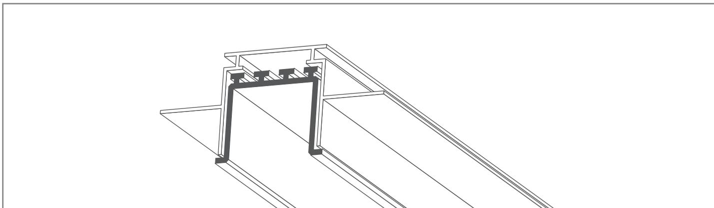
**Parts needed to mount the LOKOM extrusion**
