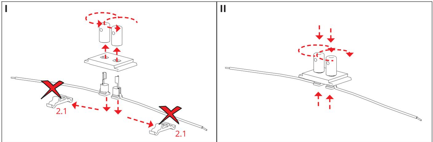
In case of installation in the GIZA-DUO-LL profile, unscrew the fastener and remove its blockades. Then fold the fastener back.
