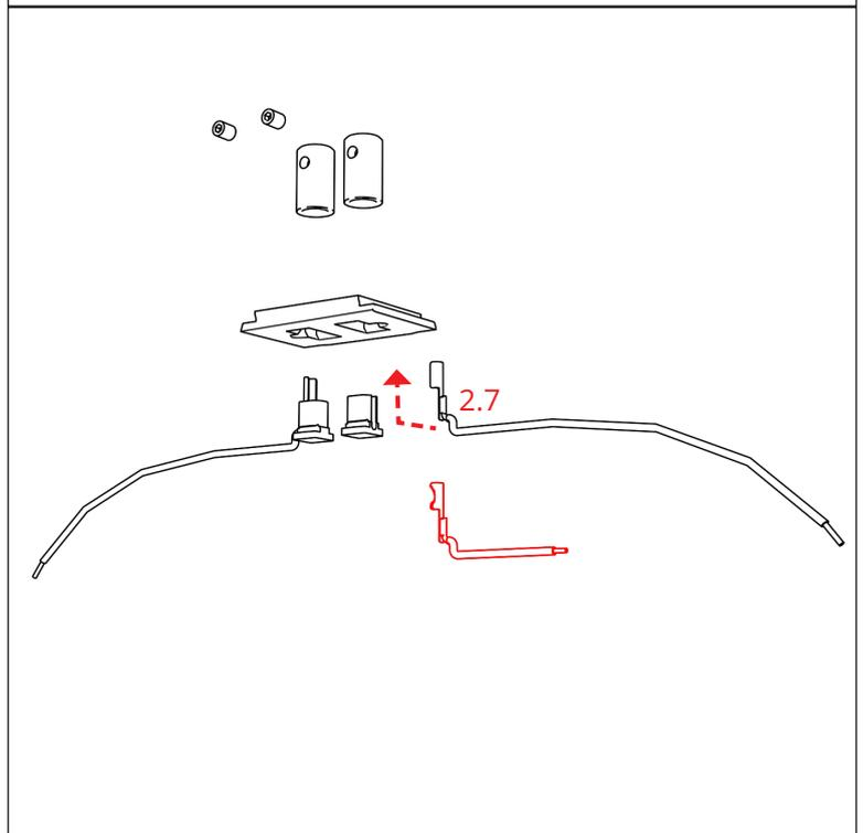
In case of damaged fastener's connector, unfold it for parts and replace damaged item.
