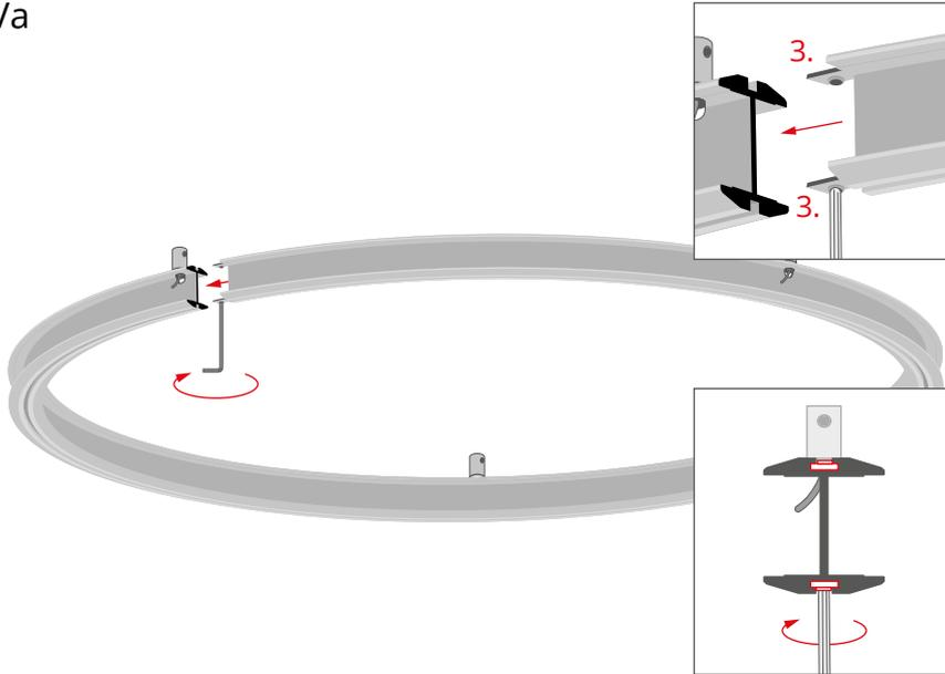
Connect the profile elements with the connectors (3) and lock them in place.
