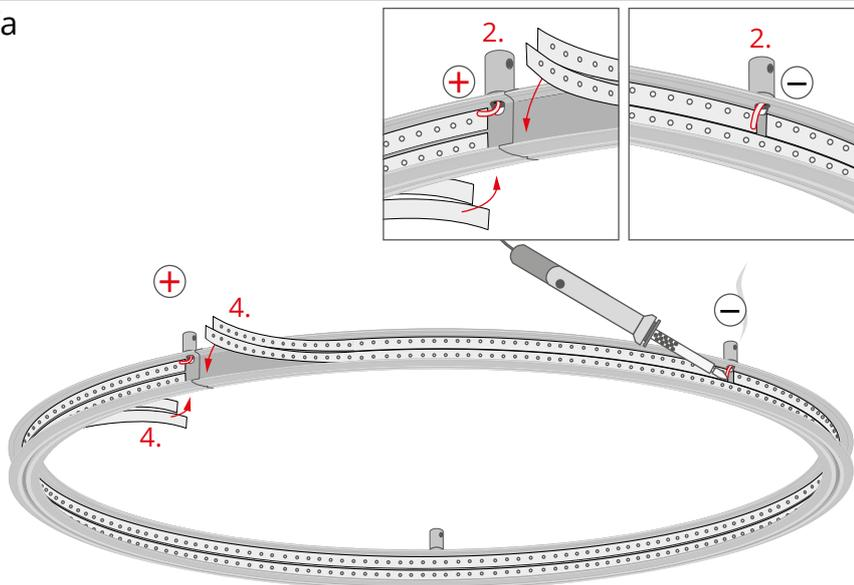
Adhere the LED tapes (4) on both sides of the profile and solder the wires from the fasteners (2) to them.
